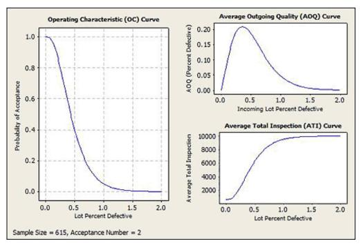
Figure: Operating Characteristic Curve, Average Outgoing Quality Curve and Average Total Inspection Curves for Single Sampling Plan
