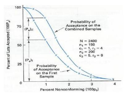
Figure: OC Curve for Double Sampling Plan
